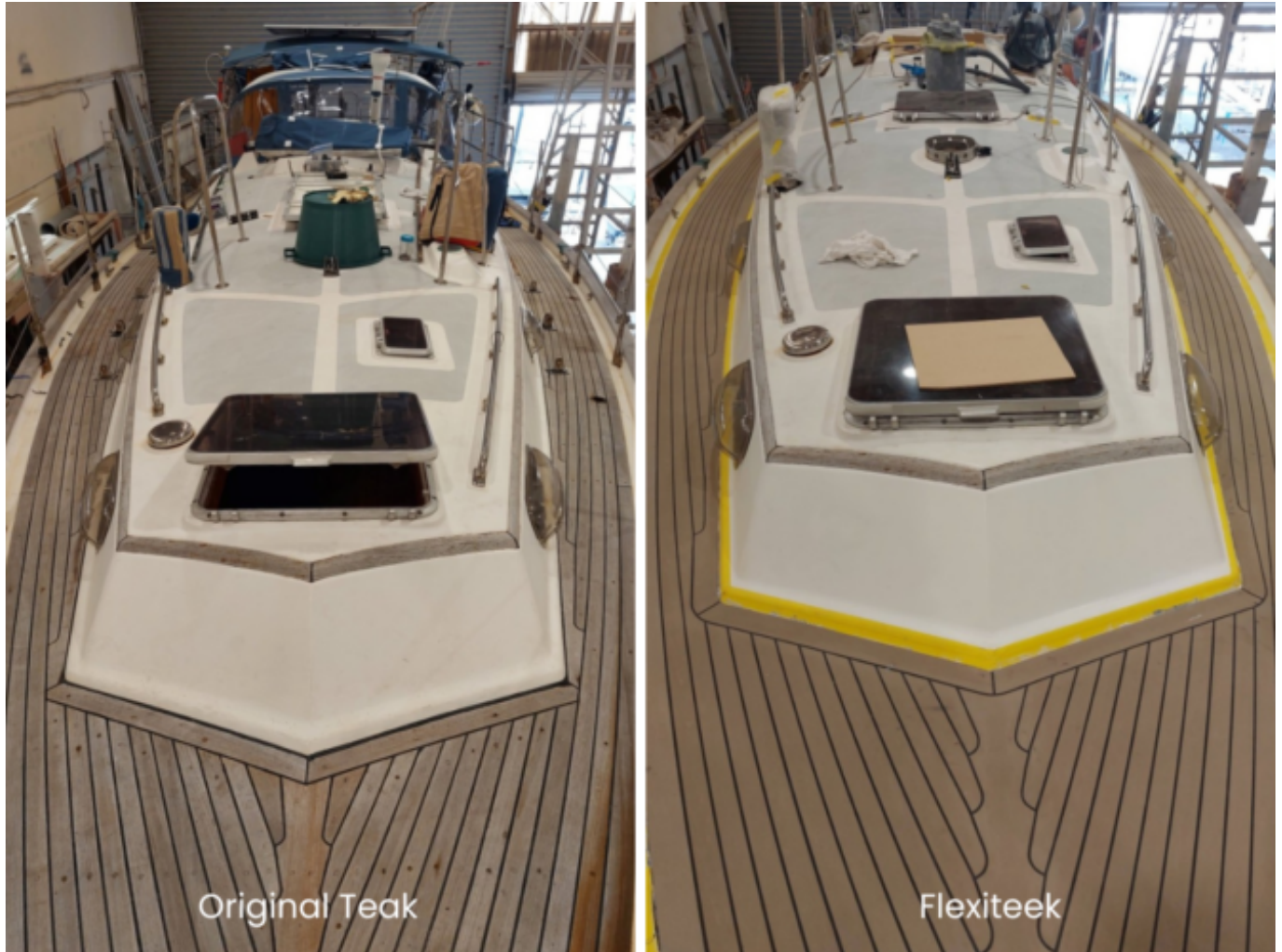
The original teak deck compared with the new Flexiteek.
