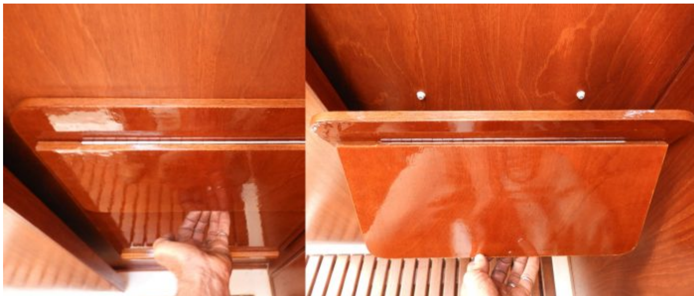
Fig.9 Deploying the fold-down step by pulling the support leg away from the bulkhead.
