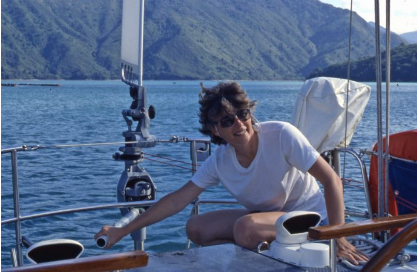
Tiller to steering emergency rudder
