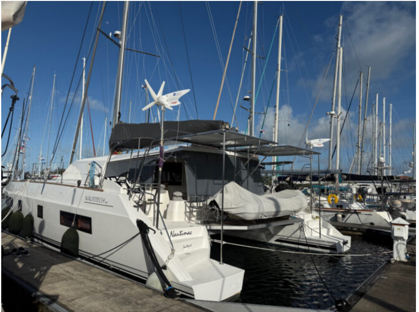
A catamaran with two wind generators — port and starboard.
