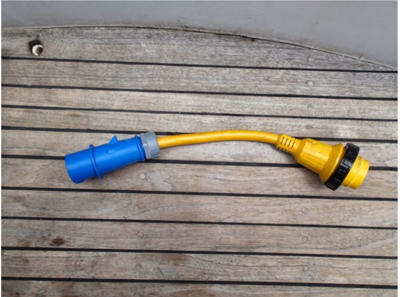
30 amp pig tail adapter was needed to convert to European power
