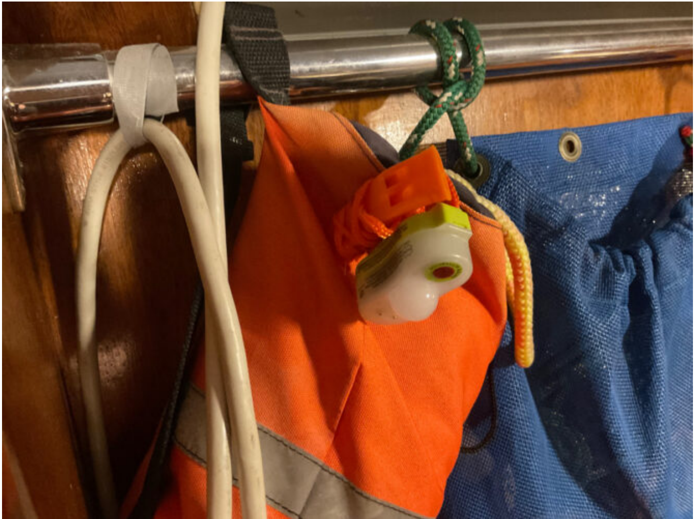
A HemiLight water activated light and whistle attached to a heaving line's case.
