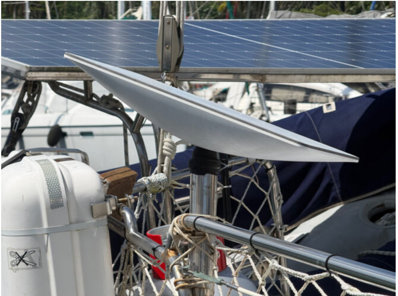
A Starlink using the classic pole stuck in a fishing rod holder mount.
