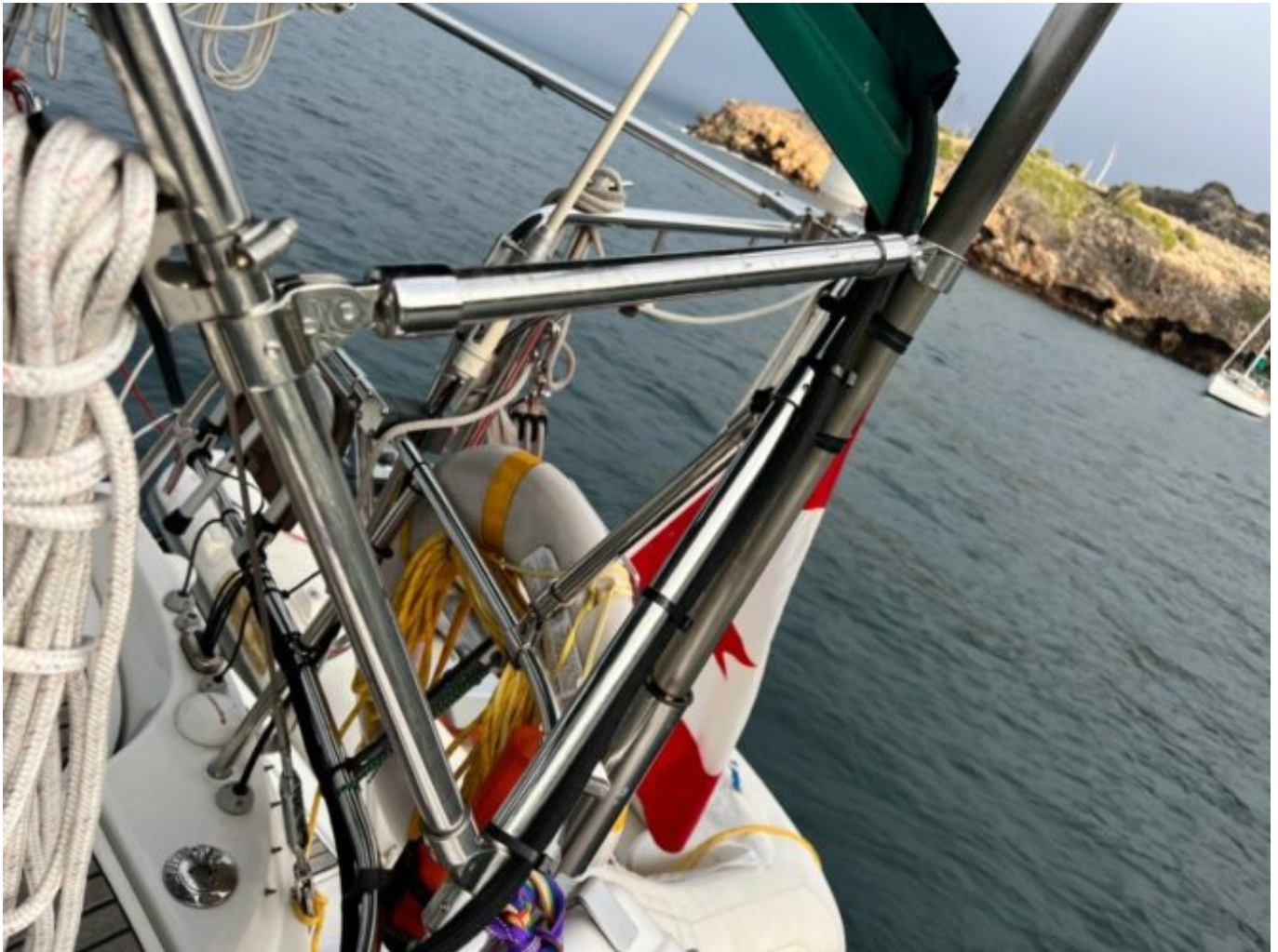
1” pipe connected to Bimini frame
